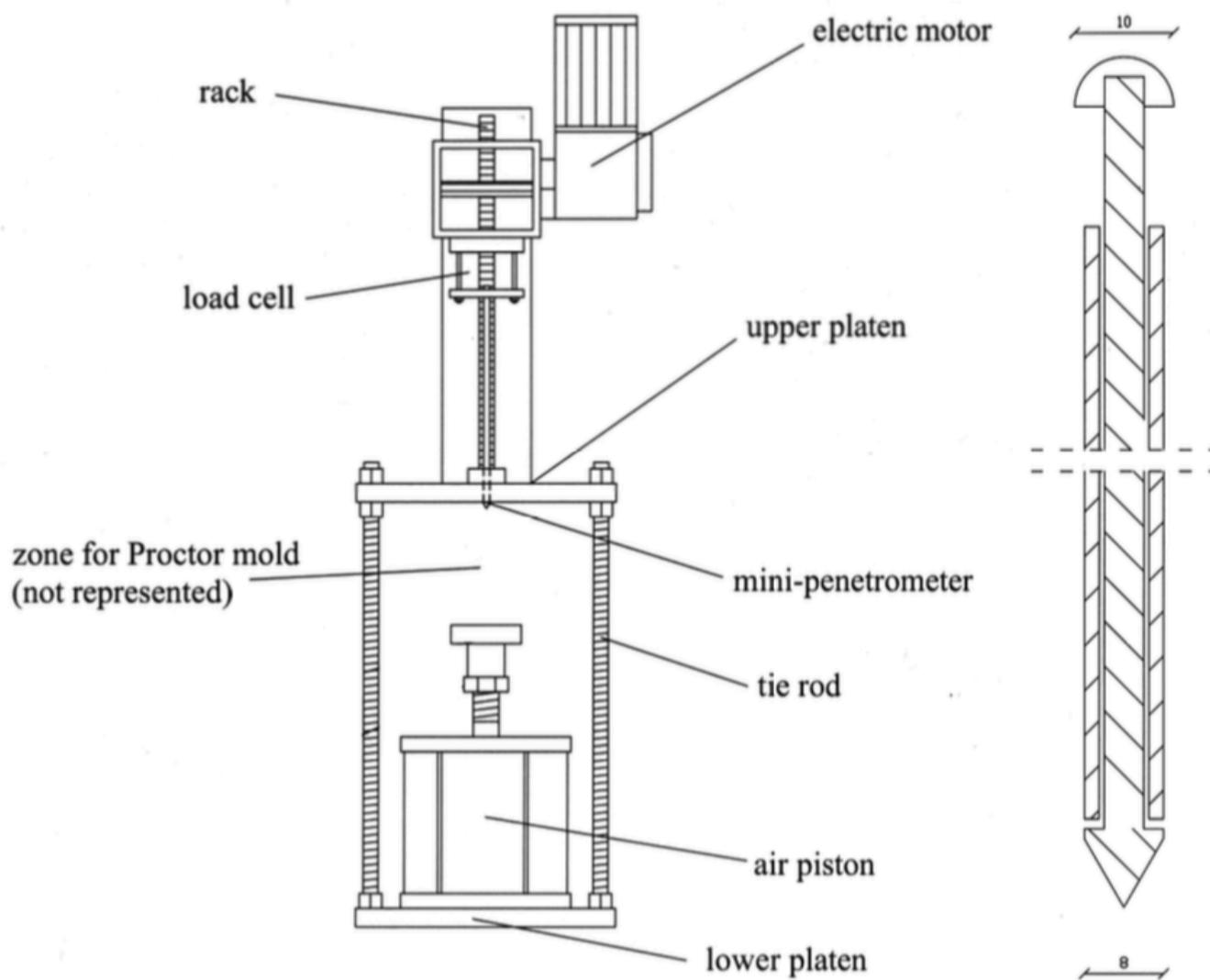
Figure 31. Scheme of equipment. On right see the detail of mini penetrometer.
