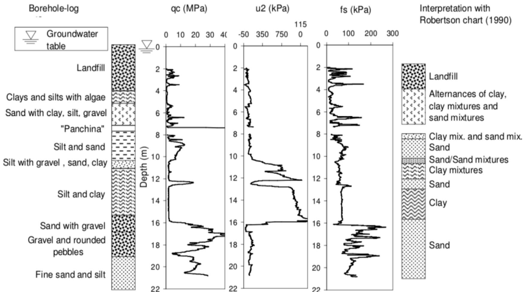
Figure 26. Site 2 (Livorno). Comparison between the CPTu carried out with the standard penetration rate (2 cm/s) and a nearby borehole-log.
