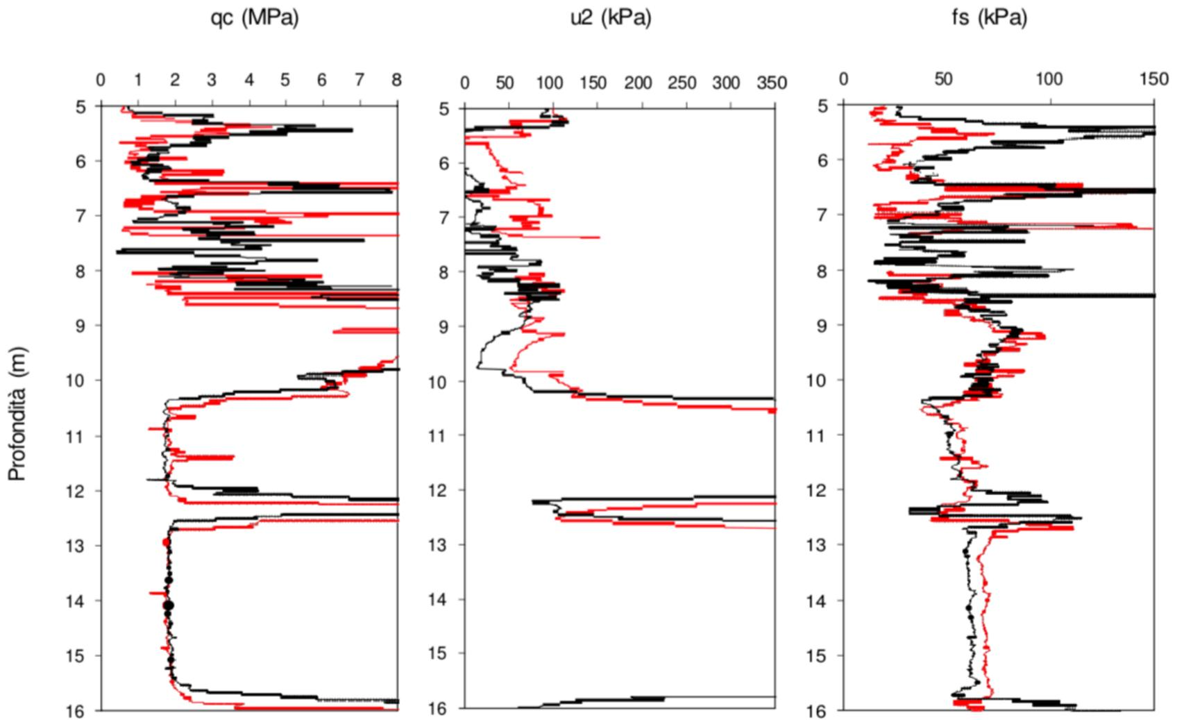
Figure 30. Livorno. Comparison between the slower rate (black line) and the standard rate (red line).
