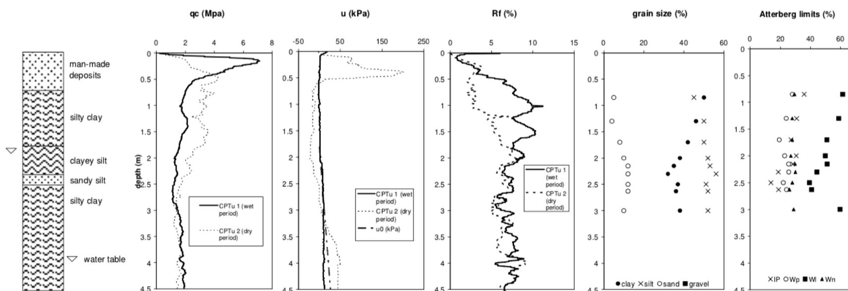
Figure 20. Scuropasso Stream alluvial fan. Soil profile and geotechnical characteristics.  $q_c$ : cone resistance;  $u_0$ : in-situ pore pressure;  $u_2$ : pore pressure measured at cone base;  $f_s$ : sleeve friction;  $R_f$ : friction ratio ( $f_s/q_c \cdot 100$ ) IP: plastic index; Wp: plastic limit; WI: liquid limit.
