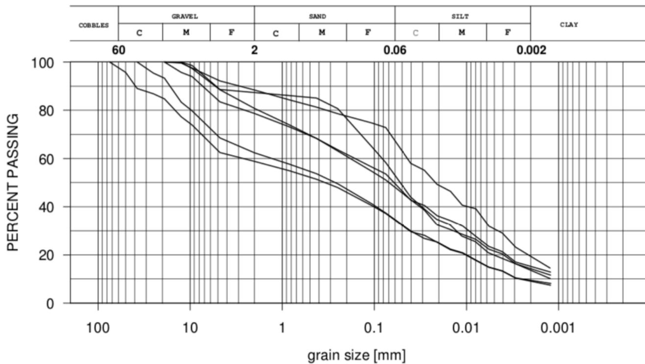
Figure 36. Grain size distribution of samples
