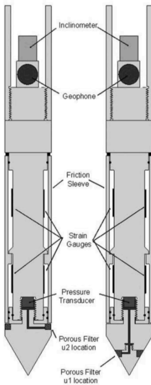
Figure 4c. Scheme of piezocone tip
