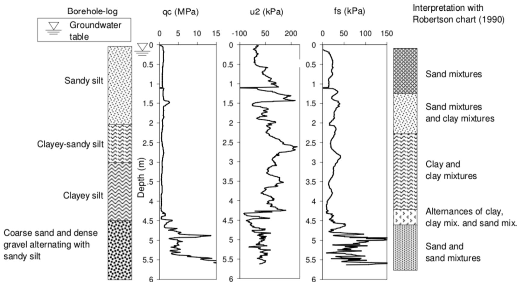
Figure 25. Site 1 (Paganico). Standard CPTu (2 cm/s) compared to a near borehole-log.
