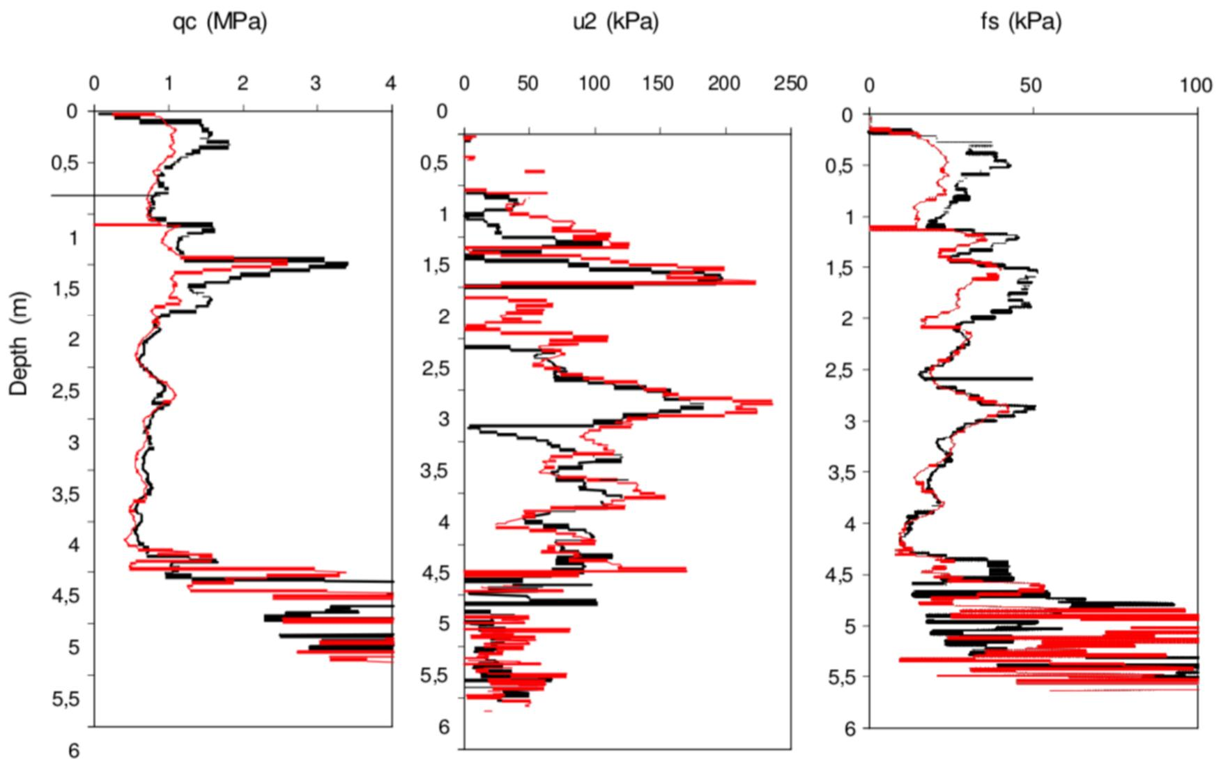
Figure 28. Paganico. Comparison of the standard rate (red line) and the slower rate (black line)
