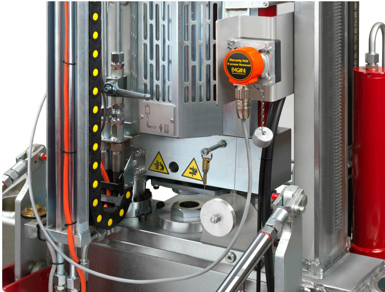
Figure 10. Example of depth logger
