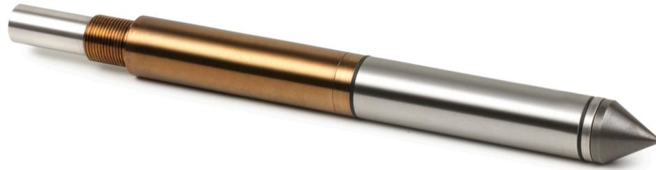
Figure 4d. Picture of CPTu tip
